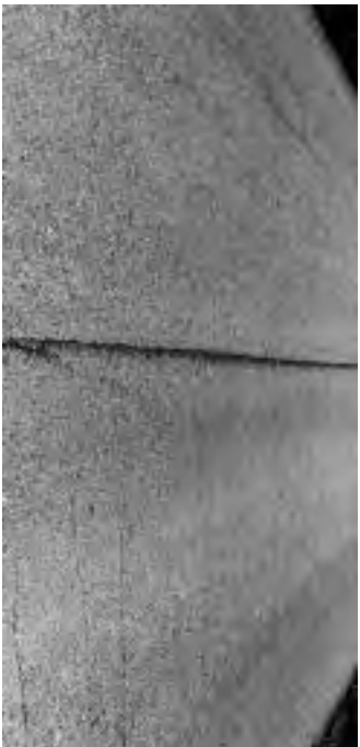
Centerline crack (still tight). ▶
