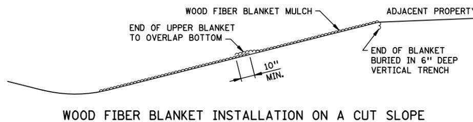
WOOD FIBER BLANKET INSTALLATION ON A CUT SLOPE
