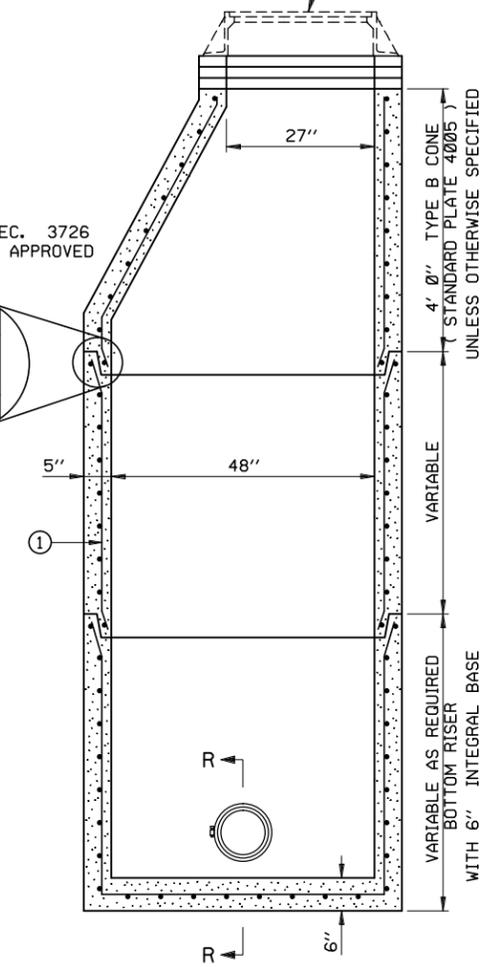
**SECTION THRU TYPICAL MANHOLE**
