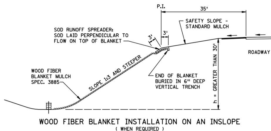
WOOD FIBER BLANKET INSTALLATION ON AN INSLOPE ( WHEN REQUIRED )
