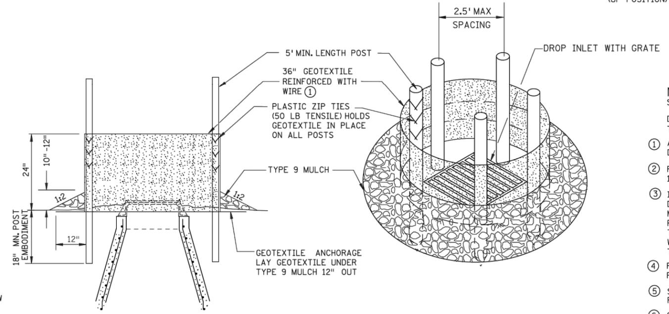
**SILT FENCE RING AND ROCK FILTER BERM**
