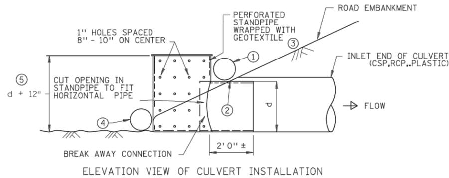
CULVERT STANDPIPE INSERT (D-RISER)
