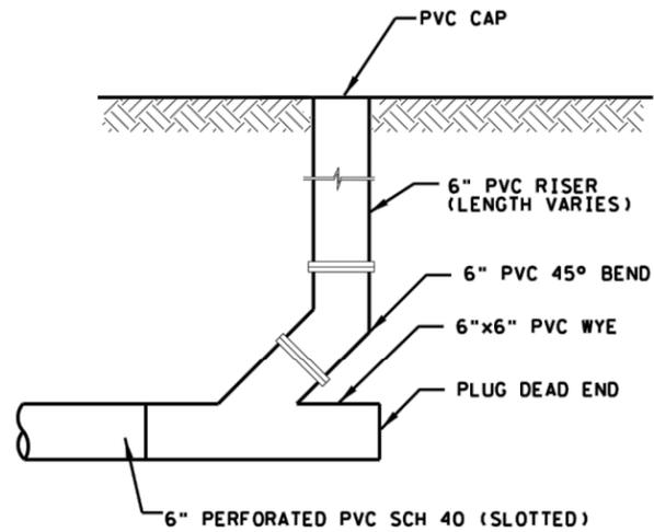
**PVC PIPE DRAIN CLEANOUT**
