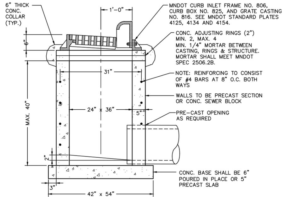
**CONSTRUCT DRAINAGE STRUCTURE DESIGN SPECIAL 1
