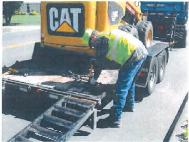
Ratcheting tie downs (grip/bend) to transport heavy equipment.
