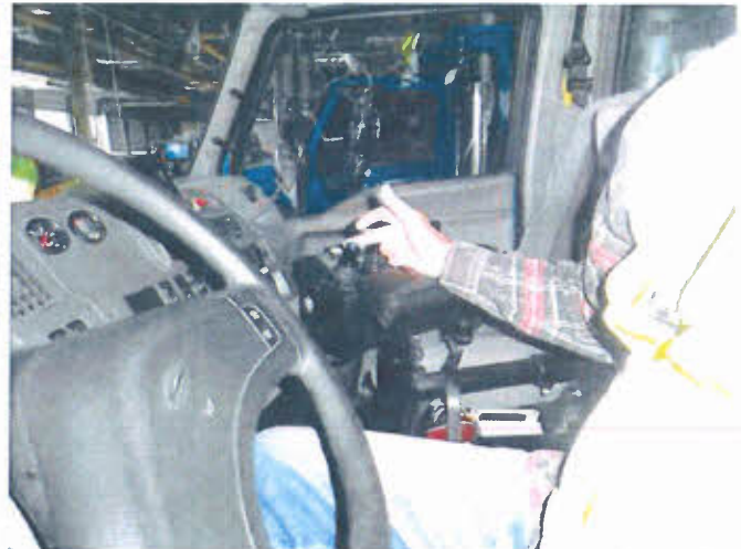
Hand operation of the control mechanism for dump box and snow plowing.
