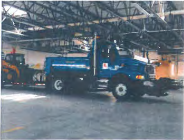
Dump truck has plow attachment for winter.
