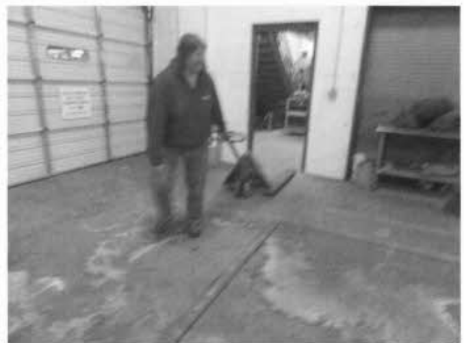
Hand pallet jack are used to move some equipment or materials in the plant.
