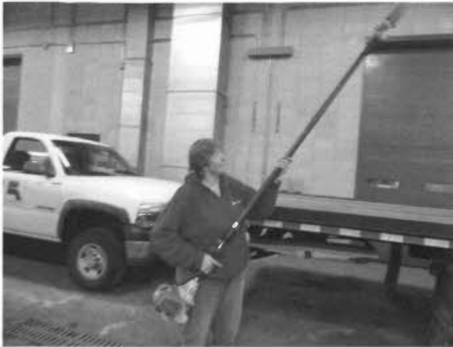
Demo of cutting branches with a _____. Weight of the saw is 20 lbs. Larger cut branches are moved by a team lift.
