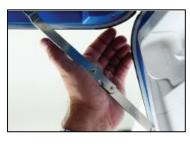
12 Use blue key to unlock tablet and slide latch to remove the tablet.
