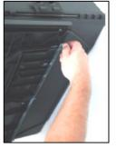
Luse the black key to unlock and open front door and press bottom of the box into place.
