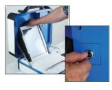
14 Turn the machine on by pressing the red power button on the back of the machine. The ballot counter will take about 7 minutes to power-up.
