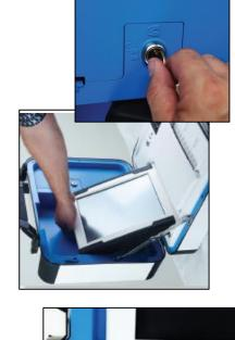
Turn the machine on by pressing the red power button on the back of counter will take about 7 the machine. The ballot minutes to power-up.
