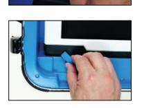
L Close the cover of the ballot counter and snap the black latches in place. You do not need to lock the case.
