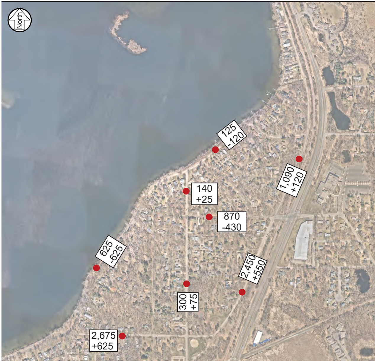
FIGURE 3: Proposed Traffic Conditions - One-way traffic north/east-bound on Bald Eagle Boulevard east of Park Avenue and Taylor Avenue and Two-way traffic on Hugo Road and Bald Eagle Avenue west of Park Avenue. (numbers indicate Average Daily Automobile Traffic)
