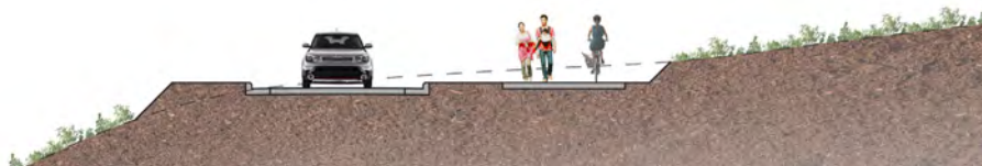
FIGURE 4: One-way roadway with trail on right.
