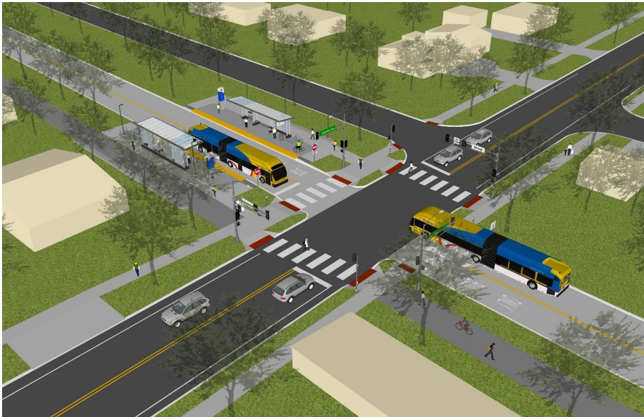
Figure 34. Visualization of typical station, trail, and dedicated BRT roadway. 118
