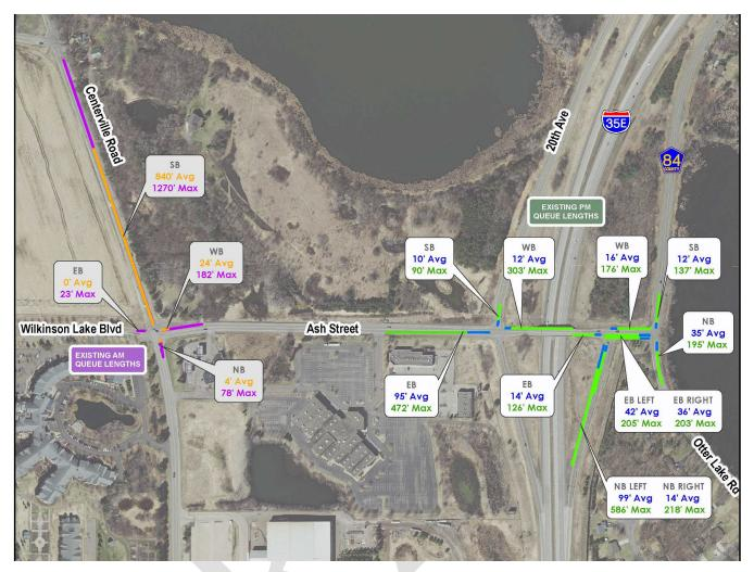
However, as illustrated in the map above, there are still queueing issues that spill between the closely-spaced intersections around the existing I-35E ramp terminals and Otter Lake Road (Anoka CSAH 84/Ramsey CSAH 60). With essentially no turn lanes provided, the single lane approaches quickly build queues that impact upstream intersections. Very long queues also occur for southbound Centerville Road traffic at the CR J intersection.
