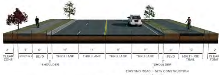
VICTORIA STREET EAST SIDE CONCEPT, TYPICAL SECTION A - A
