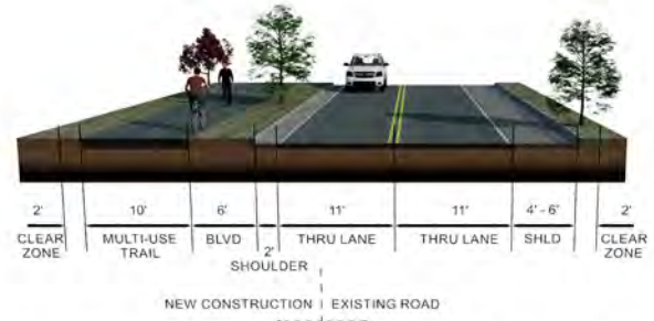
VICTORIA STREET WEST SIDE CONCEPT, TYPICAL SECTION B - B
