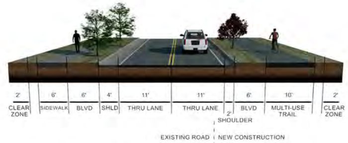
VICTORIA STREET EAST SIDE CONCEPT, TYPICAL SECTION B - B
