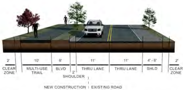
VICTORIA STREET WEST SIDE CONCEPT, TYPICAL SECTION D - D
