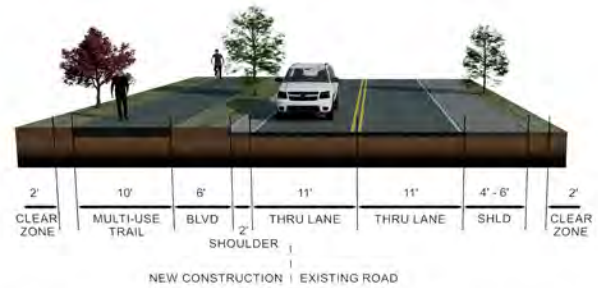
VICTORIA STREET WEST SIDE CONCEPT, TYPICAL SECTION D - D
