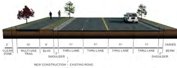
VICTORIA STREET WEST SIDE CONCEPT, TYPICAL SECTION A - A
