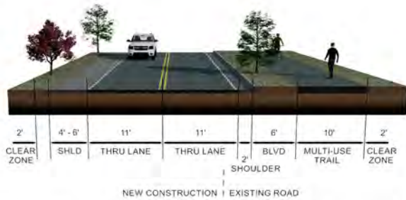
VICTORIA STREET EAST SIDE CONCEPT, TYPICAL SECTION D - D
