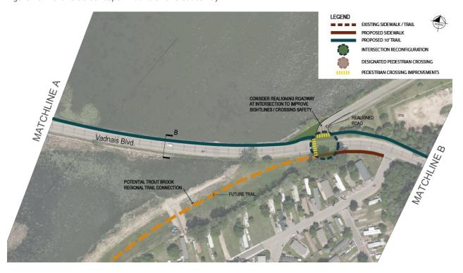
Figure 17. Typical Section B – Vadnais Lake Causeway, North Side Concept
